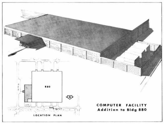
ARTIST'S CONCEPTION of the new addition to Bldg. 880. Enclosed in the screen block wall on the right are cooling towers for the air conditioning system. Inset on the lower left shows the location of the new structure.
